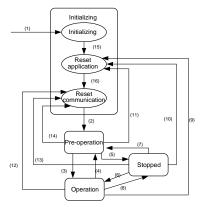
Figure 3-3 NMT state diagram
